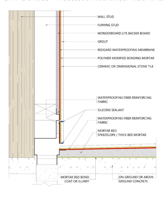
NOTE: Illustration shows the necessary components of the tile installation method, including the substrate. This has not been drawn to scale. It is intended to clearly identify and label each component and its placement in the assembly.
