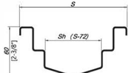
(Sv) - Standard channel with v-shaped bottom
