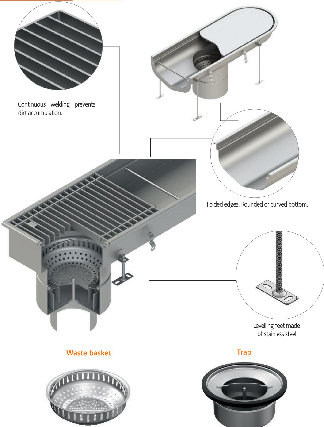
Deep pressed, without welding, single hygienic element for effective cleaning and removal of solid wastes.
