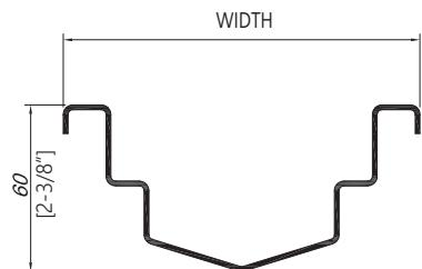
**Sv16V1: 16" WIDE STAINLESS STEEL TRENCH DRAIN WITH "V"-SHAPE BOTTOM & VERTICAL OUTLET**
