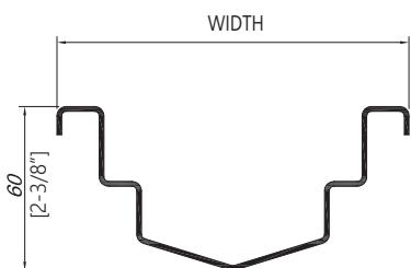
**Sv6H1: 6" WIDE PRE-SLOPED TRENCH DRAIN WITH "V"-SHAPE BOTTOM & HORIZONTAL OUTLET**
