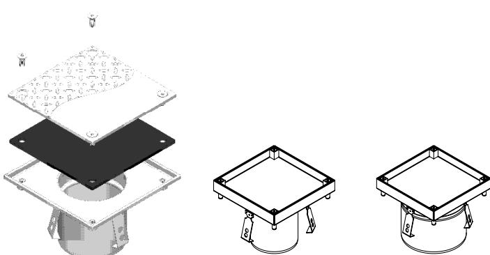
These sewage system elements are widely applied in industrial facilities (chemical, food, pharmaceutical plants etc.). Use of a rodding eye allows quick access to the underfloor area and easy cleaning.
