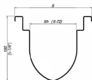
(Su) - Narrow standard channel with rounded u-shape bottom
